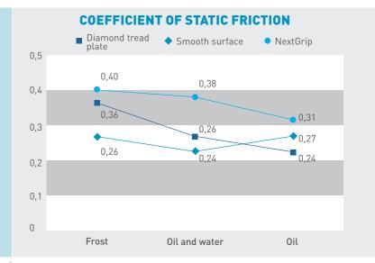
\*Tests where conducted on 0.100 inch aluminum.
