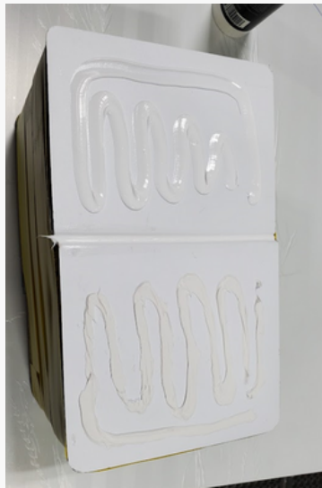
Sealant at time of application
